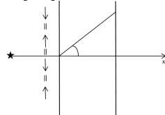
The intensity of the interference pattern measured on a distant screen, at an angle  $\theta = n\lambda/w$  to the x-axis is
